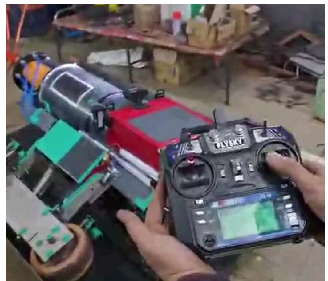
Fig.4.4 : Show the Remote operational capabilities of M-TBM
